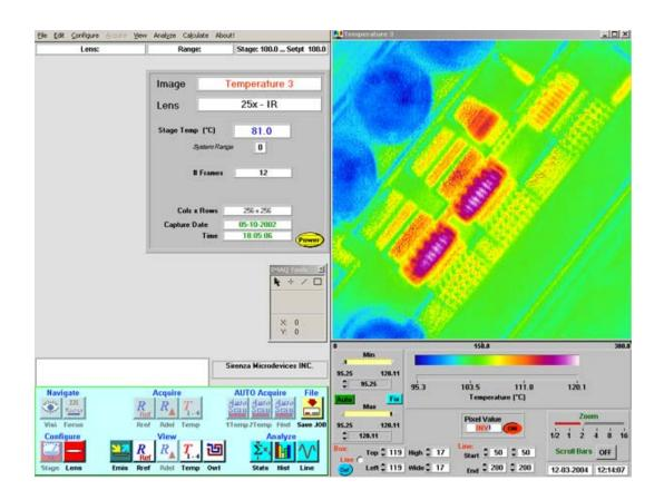
Figure 2: Infrared Thermal Image of SGA-6586Z, Vd = 4.50V, Id = 80.2mA, Tlead = 84.5°C
