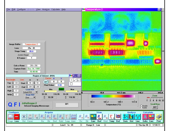
Figure 1: Infrared Thermal Image of SGA-6486, Vd = 4.65V, Id = 80.3mA, Tlead = 85.5°C
