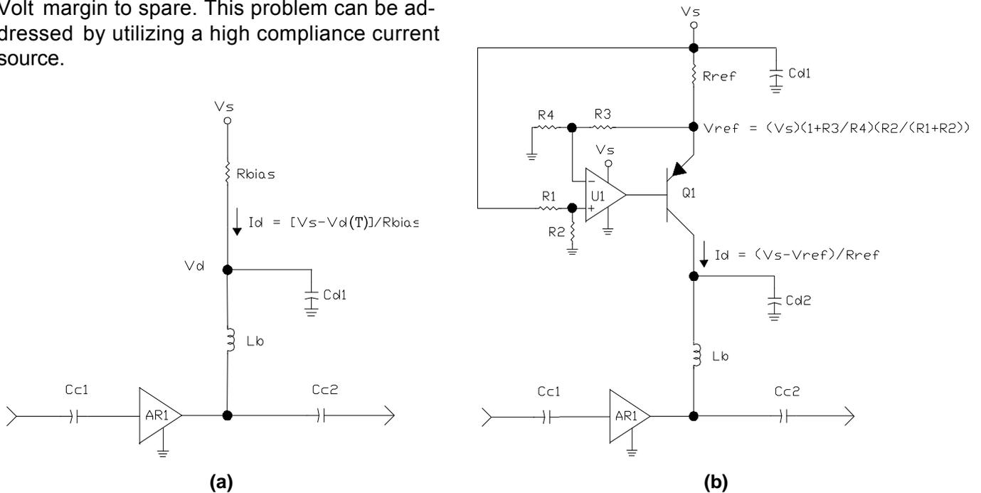
**Figure 1 : (a) Standard Gain Block Passive Bias Circuit
