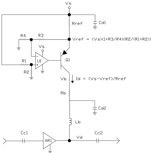
In schematic at left,  $L_b = 1.5 \mu\text{H}$ .  $C_{c1,2} = .01 \mu\text{F}$ .  $C_{d1} = 1 \mu\text{F}$  tantalum  $C_{d2} = 2 \times .01 \mu\text{F}$  (ceramic chip) +  $1 \times 22 \mu\text{F}$  tantalum. The dc conditions per schematic at left were measured per the table below.
