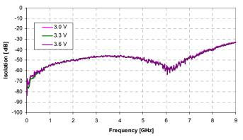
Figure 12. Isolation: RFC to Isolated Port @ 25 °C
