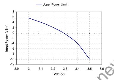
To allow for sustained operation under any load VSWR condition, max power should be kept 6dB lower than max power in 50 Ohm.
