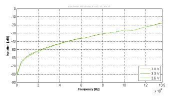
Figure 13. Isolation: RFC to Isolated Port @ 3.3V
