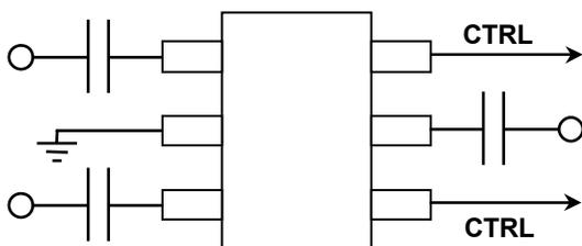
Consider the typical SPDT in Figure 2. Every RF interface is capacitor-coupled. Now tie the ground
