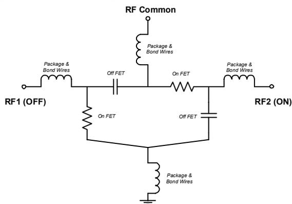
Low power switches (P1dB up to +27 dBm) use transistors with thresholds of 0.8 volts. Low-voltage CMOS logic drive them directly. In higher power switches (P1dB up to +30dBm), a 3-volt control span is insufficient for signal swing. Once again, UltraCMOS technology has a solution because any CMOS function is easily integrated.
