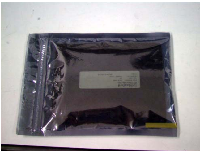
Static shielded bags are typically dark silver in color, and may (or may not) have the ziplock mechanism on them. They should be marked as "static shielded" somewhere on the surface of the bag. These are highly recommended for transporting static sensitive devices.
