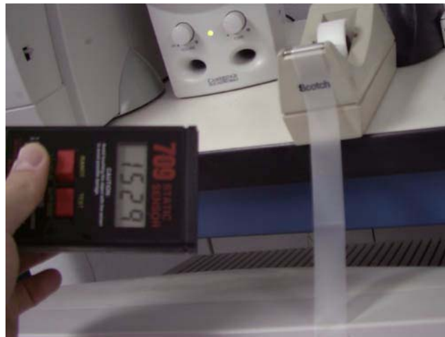
Transparent tape (i.e. "Scotch Tape") generates large amounts of static charge as it is unwound from the roll. The meter shows the high level of static charge carried on the surface of the tape, which is then discharged through the item being taped.
