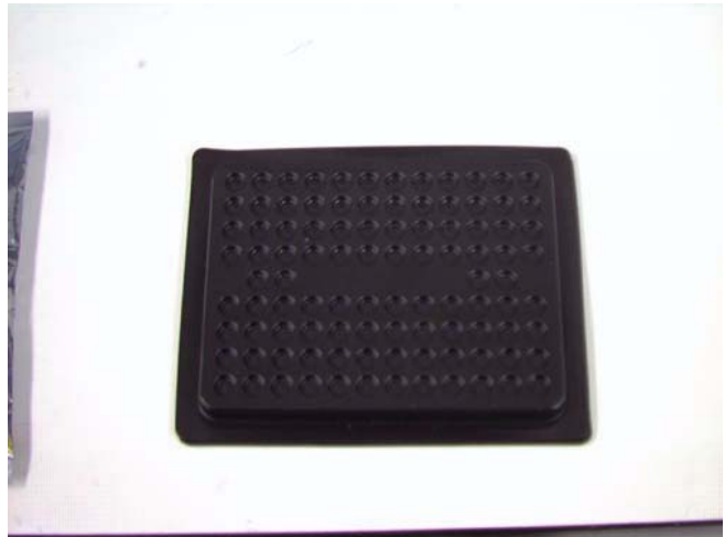
Electrically conductive chip trays are good for storing or transporting static sensitive materials when used with shielding bags. The conductive surface acts like a Faraday cage, so static charges are conducted around the outside of the tray and dissipated to ground without going through the devices.
