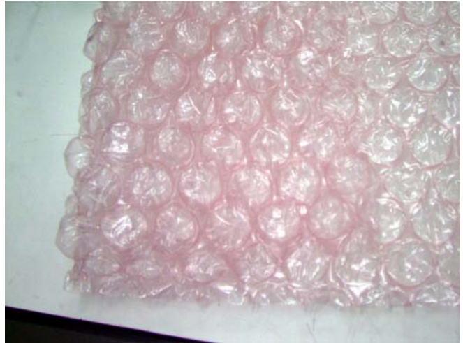
Plastic bubble wrap is also not a good packaging material. It is also an insulator, and will retain static charges for a long period of time.
