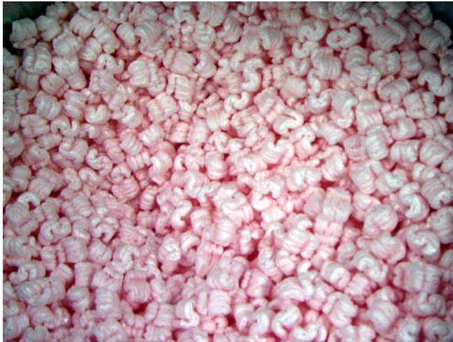
Styrofoam peanuts are not a good material to use when shipping static sensitive parts. Styrofoam is an insulator, and will retain static charges for a long period of time.
