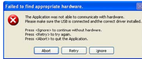
Figure 8. Warning that displays when the programming tool starts with no device connected
