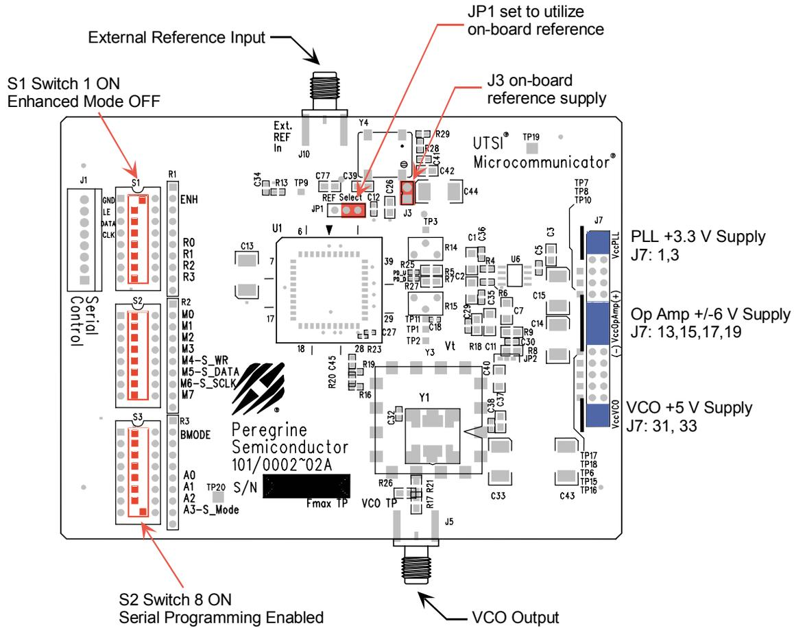
**Figure 3. Jumper Setting to Disable On-board Reference.**
