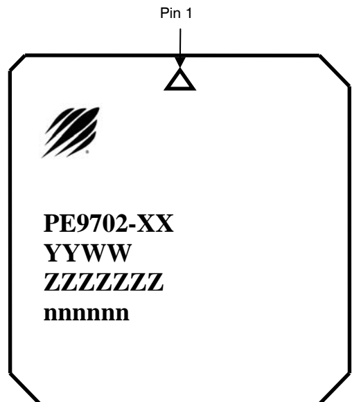
Figure 8. Top Marking Specifications
