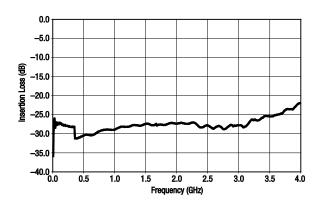
**Figure 4. Input Return Loss vs Frequency**
