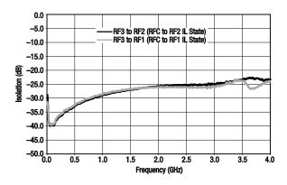
Figure 7. Port-to-Port Isolation vs Frequency
