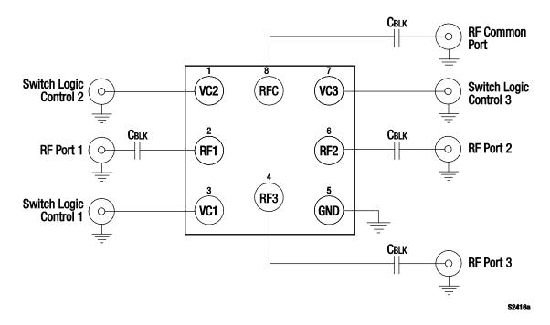
Figure 8. SKY13386-000 Evaluation Board Schematic
