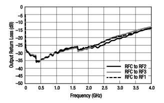
Figure 5. Output Return Loss vs Frequency
