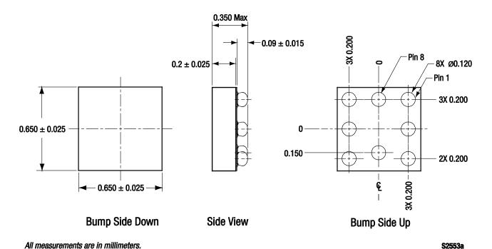
Figure 10. SKY13386-000 8-Bump CSP Package Dimensions
