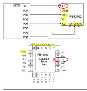
**Parallel programming (Figures 1 and 2):** The desired attenuation level is programmed directly onto each control pin (direct-parallel) or indirectly latched onto each control pin (latched-parallel).
