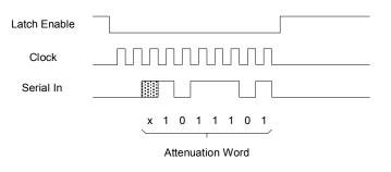
The main advantage of serial control is reduced routing complexity. For PE43702, control lines have been reduced from seven in direct-parallel mode to three in serial mode. Isolation considerations are therefore also simplified. The main disadvantage of serial control is slower speed; however, clock speeds in modern electronic systems are so fast that this is often not a problem.
