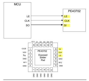
**Serial programming**: Attenuation is programmed within a one-byte Attenuation Word, least significant bit first.
