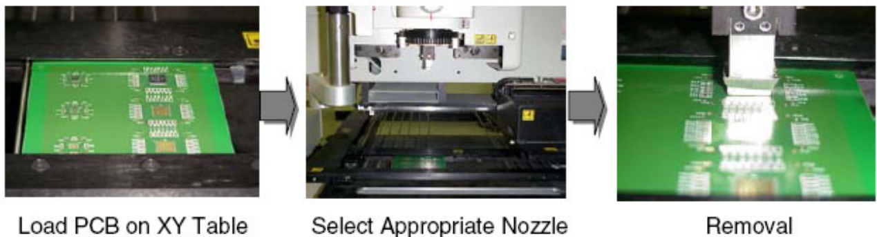
Figure 4. Typical Package Rework Station and Process
