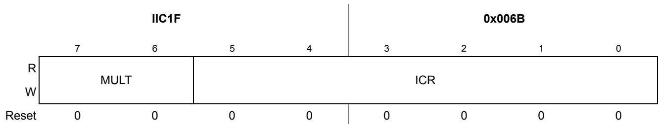
Figure 12-3. IIC Frequency Divider Register (IIC1F)
