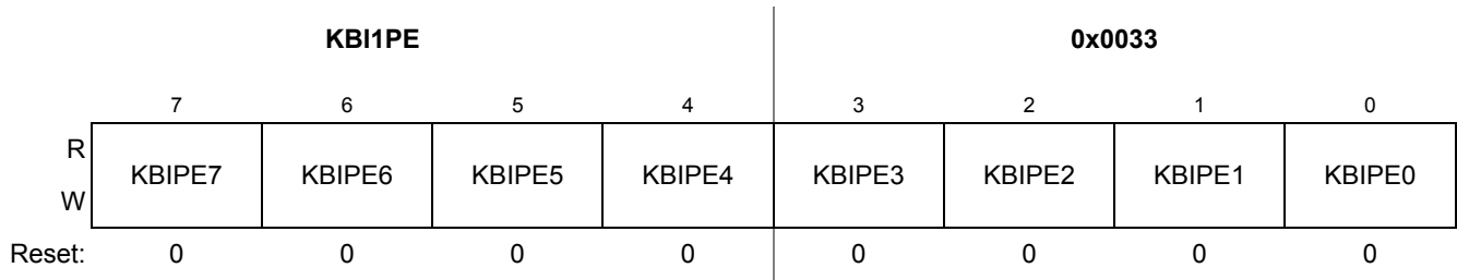
Figure 11-3. KBI1 Interrupt Pin Select Register (KBI1PE)
