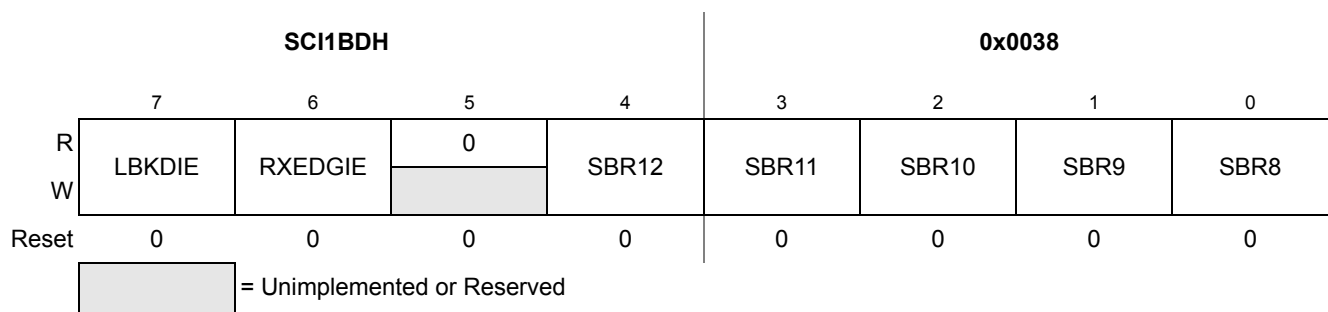
Figure 13-4. SCI Baud Rate Register High (SCI1BDH)
