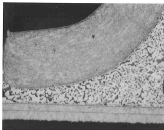
Figure 17. Close-up View of the Solder Joint Cross-section at the Lead to PCB Bond Pad
