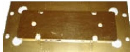
Figure 5. Typical PCB with Coin Attached to the Backside
