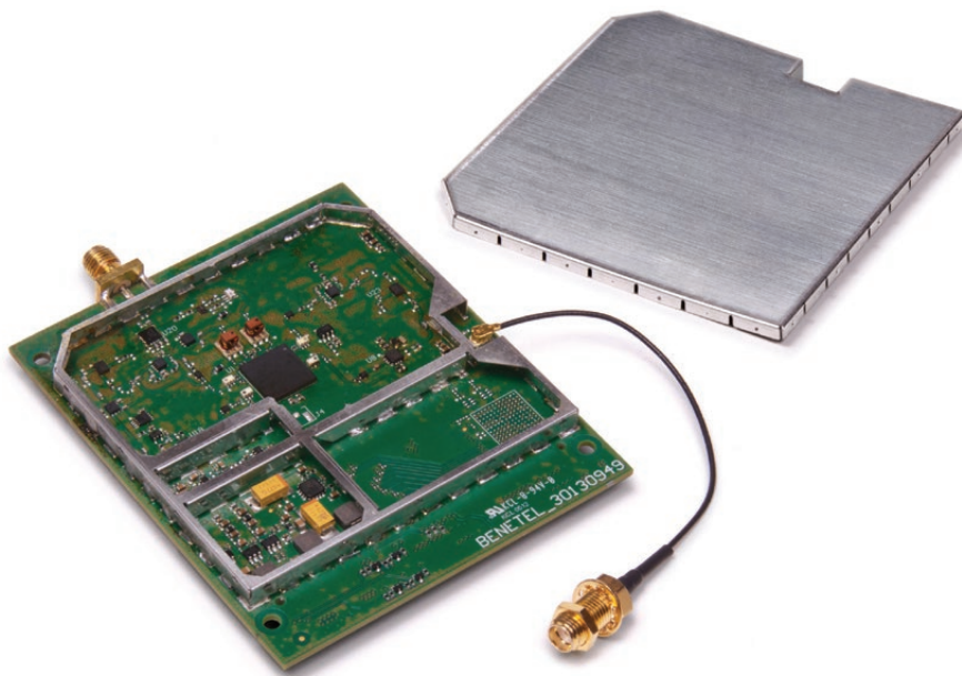
LTE-FDD/TDD and W-CDMA (HSPA+) Capable RF Module
