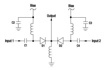
Figure 2. Typical MIS Capacitor Application Circuit
