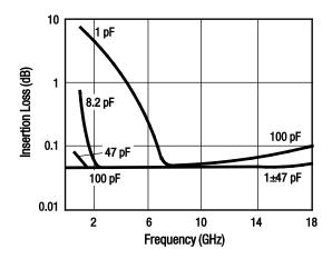
Figure 1. Typical Insertion Loss vs Frequency (50  $\Omega$  System)
