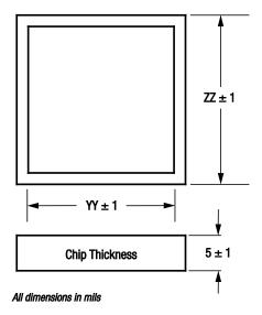
**Figure 3. MIS Capacitor Chip Dimensions**
