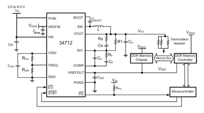
Figure 1. Application diagram for 34712
