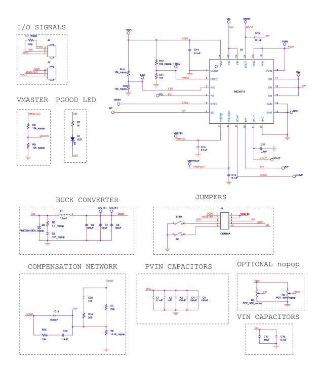
Figure 3. 34712 Schematic
