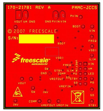
Figure 6. PCB Layout Bottom Layer
