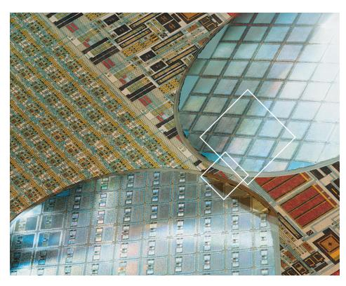
**SMARTMOS** technology, in combination with HDTMOS and discrete FETs, for very high current capability, is Freescale's predominant process technology, which combines precision analog, high voltage, high current power capabilities and high speed CMOS in a single package.
