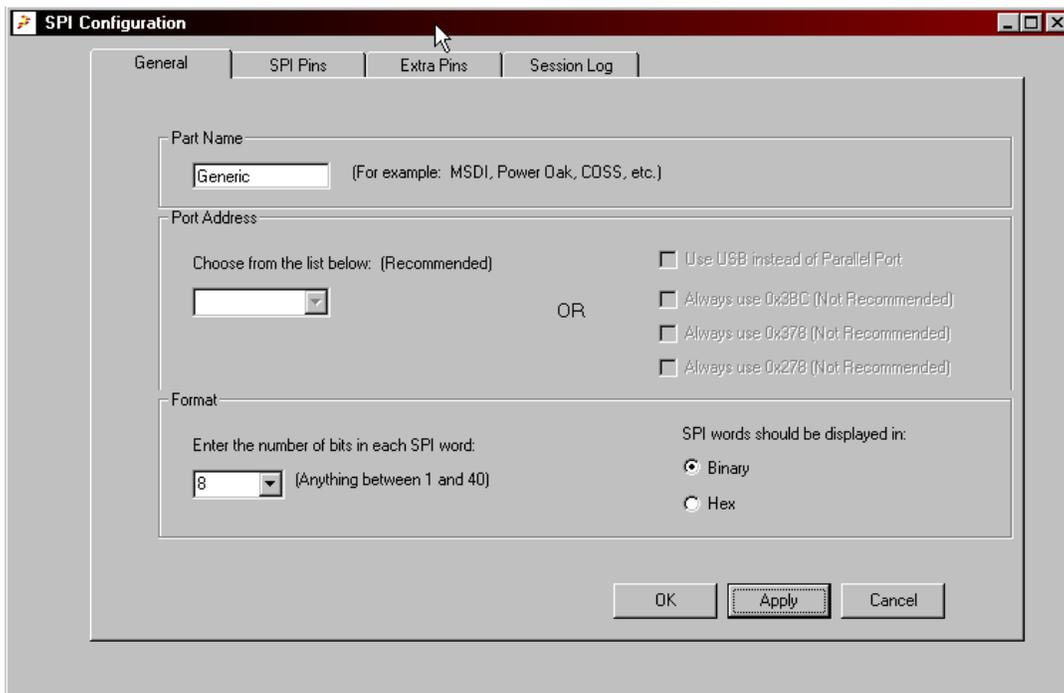
The major difference between this screen and that of SPIGen version 4.0.0, is the addition of the **“Use USB instead of Parallel Port”** check box. When this box is checked, and stays checked, it indicates two things:
