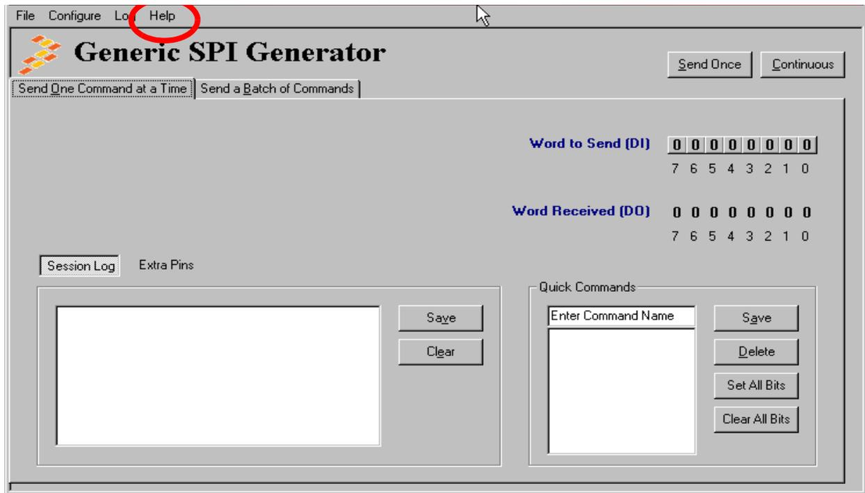
Once SPIGen is launched, the initial Window, shown above, called the “Not Configured” screen appears. At this point, the SPIGen program is not connected to either the parallel port or the USB port of the user's computer.
