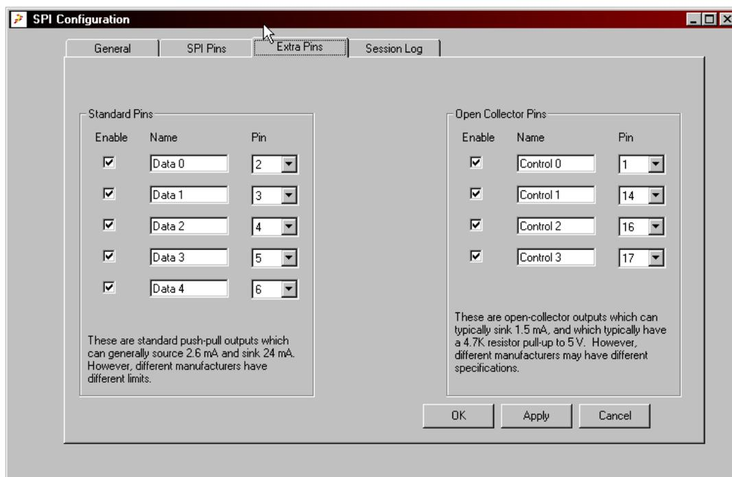
This screen differs significantly from the Extra Pins screen in the Parallel Port mode. While there are the same nine outputs, Data 0 - Data 4 and Control 0 - Control 3, there is no selection of which pins these signals are assigned to. In the USB to SPI hardware, there is a jumper mapping of these signals to pins on the DB-25 connector, so essentially the same customization is available except it is in hardware rather than software.
