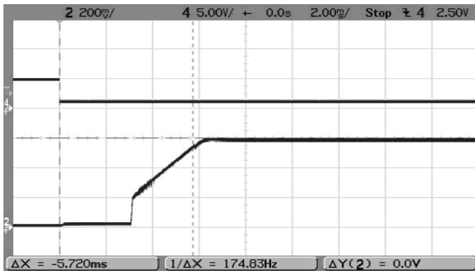
On/Off Enable Startup Delay (Vin=12V, Vout=0.591V, Iout=3A, Load=0) Trace 4=Enable In, Trace2=Vout
