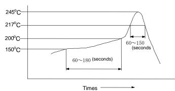
\*Do not vibrate for the products on reflow.
