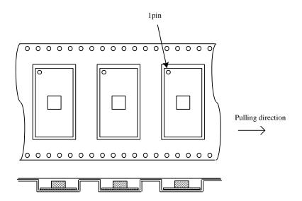
The module is located such as parts in upper side and PCB in lower side.
