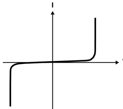
FIGURE 1. V-I CHARACTERISTICS OF A MOV
