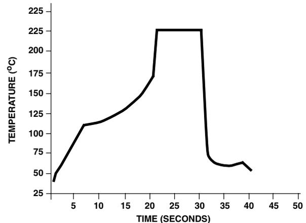
**FIGURE 7. TYPICAL TEMPERATURE PROFILE**
