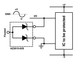
Fig. 3 Bidirectional Protection
