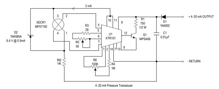
Figure 2. Schematic Diagram
