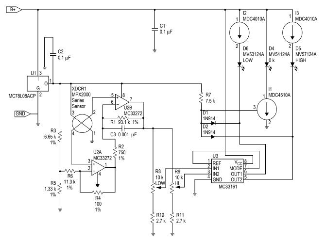
Figure 5. An Inexpensive Three-Segment Processor Monitor
