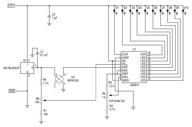
Figure 3. MPX5100 Bar Graph Pressure Gauge
