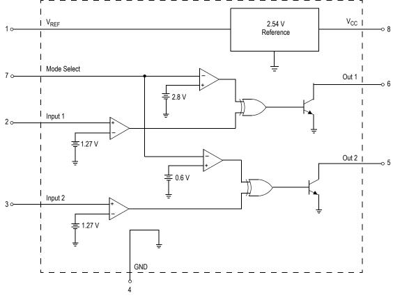
Figure 6. MC33161 Block Diagram
