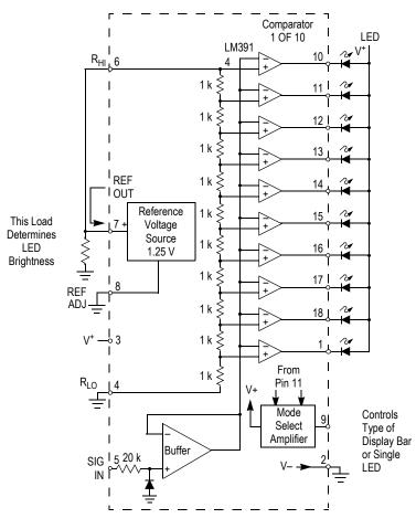
Figure 2. LM3914 Block Diagram
