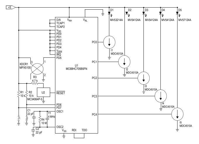
Figure 4. Microcomputer Bar Graph Pressure Gauge
