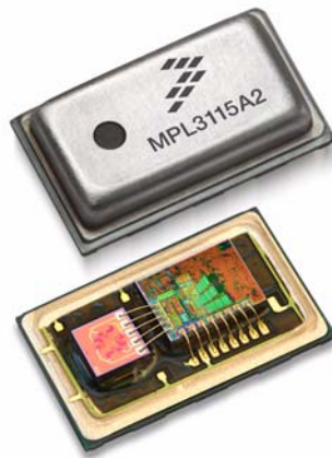
Figure 2. Zero-pressure reference (vacuum pressure) sealed inside the reference chamber
