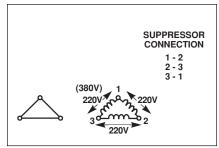
Figure 5b. 3 Phase 220V or 380V, ungrounded electrical connection
