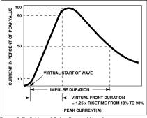
Figure 2. Definition of Pulse Current Waveform
