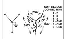
Figure 5e. 3-Phase 120V/208V, 4-Wire electrical connection
