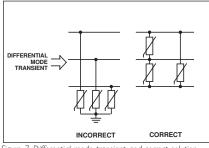
Figure 7. Differential mode transient and correct solution
