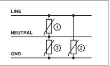
Figure 3a. Single phase electrical connection
