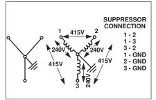
Figure 5f. 3-Phase 240V/415V electrical connection
