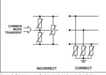
Figure 6. Common mode transient and correct solution
