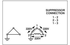
Figure 5c. 3 Phase 220V, I Phase ground electrical connection
