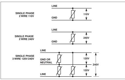
Figure 4. More single phase electrical connections
