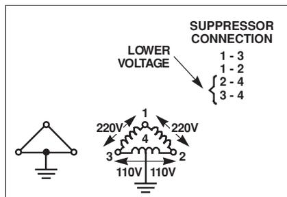
Figure 5d. 3-Phase 220V electrical connection
