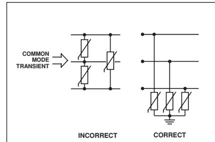
Figure 6. Common mode transient and correct solution
