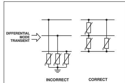
Figure 7. Differential mode transient and correct solution
