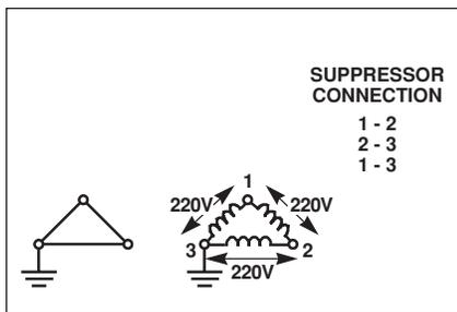
Figure 5c. 3 Phase 220V, 1 Phase ground electrical connection
