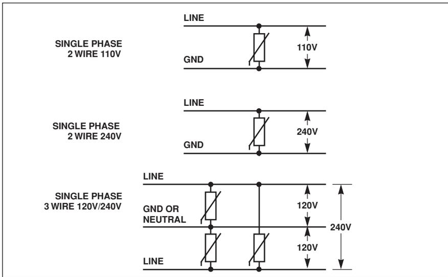
Figure 4. More single phase electrical connections
