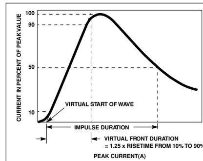
Figure 2. Definition of Pulse Current Waveform
