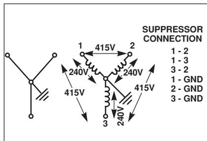
Figure 5f. 3-Phase 240V/415V electrical connection
