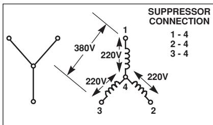
Figure 5a. 3-Phase 220V/380V, underground electrical connection
