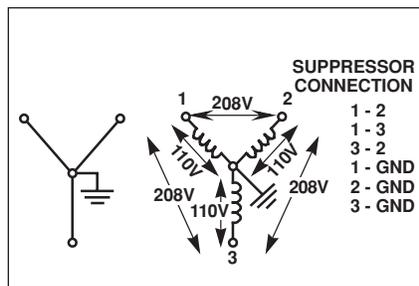
Figure 5e. 3-Phase 120V/208V, 4-Wire electrical connection
