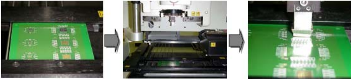
Figure 13. QFN Package Removal Process
