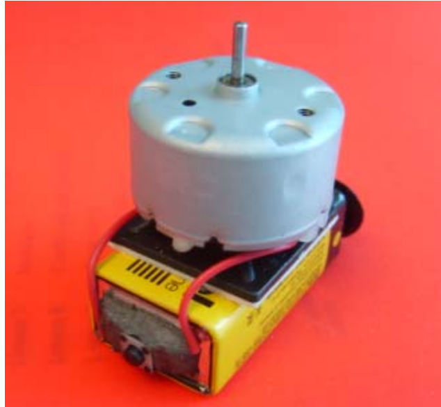
Figure 4. DC Motor used for Vibration Analysis
