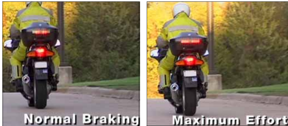
Figure 5. g-Sensor Brake Lamp Output Comparison
