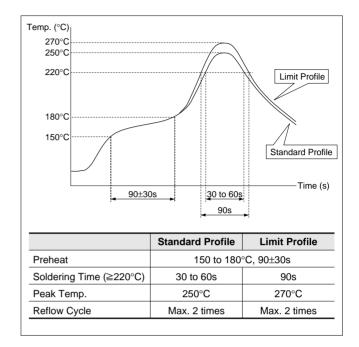
(3) There may be a risk of unexpected failures (tombstone, insufficient solder-wetting, etc.) in the mounting process, caused by the mounting conditions. Please make sure that this product is correctly mounted under specified mounting conditions.
