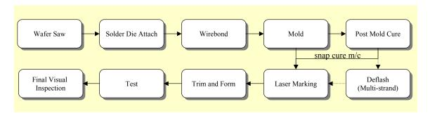
Figure 4. HSOP Process Flow Map
