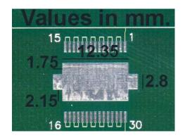
Figure 6. 30Id HSOP Exposed Pad Dimensions
