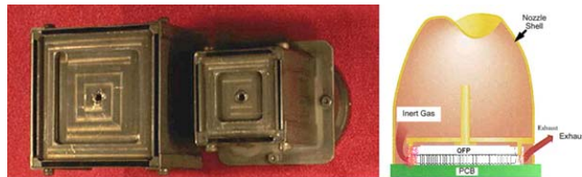
Figure 17. Examples of Typical QFP Heating Nozzles
