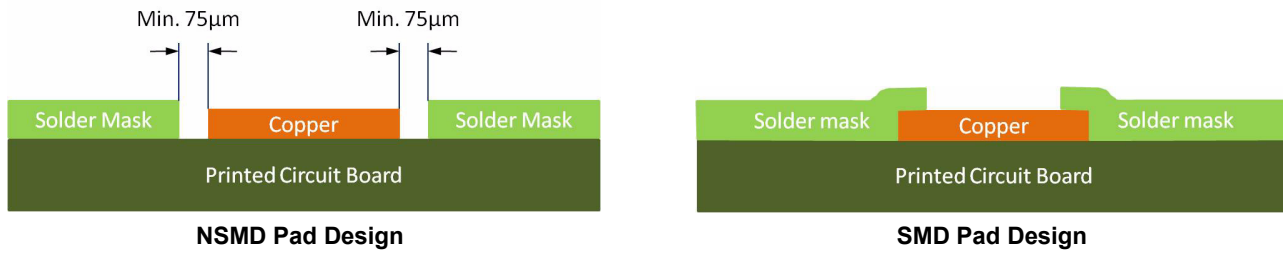
Figure 16. NSMD and SMD Pad Designs
