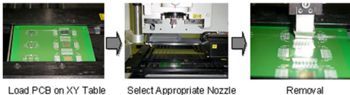
Figure 32. Package Removal Process
