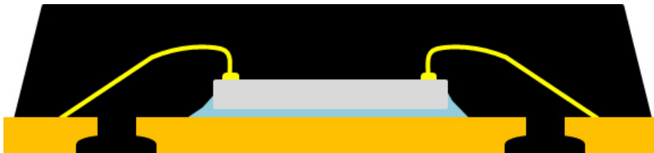
Figure 3. Punch QFN (Cross-section View)
