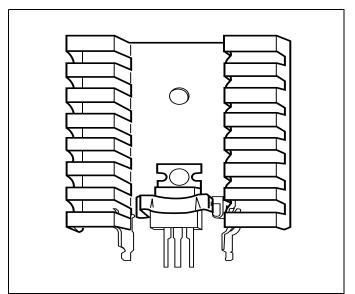
Figure AN1004.11 Typical Heat Sink Using Clips
