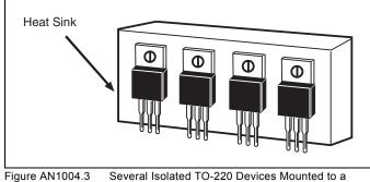
igure AN1004.3 Several Isolated TO-220 Devices Mounted to a Common Heat Sink
