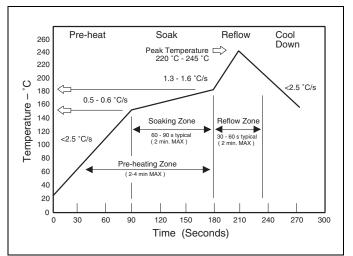
Figure AN1004.12 Reflow Soldering with Pre-heating
