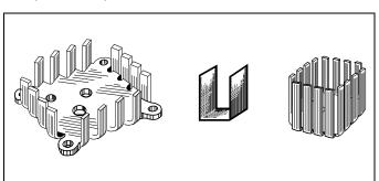
Figure AN1004.4 Examples of PC Board Mounts
