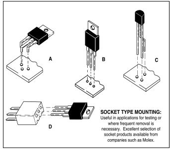
Figure AN1004.1 Component Mounting
