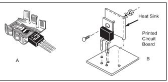
Figure AN1004.5 Vertical Mount Heat Sink
