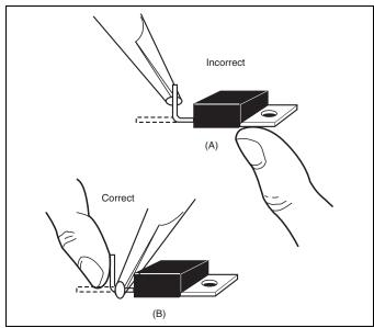
Figure AN1004.2 Lead Bending Method
