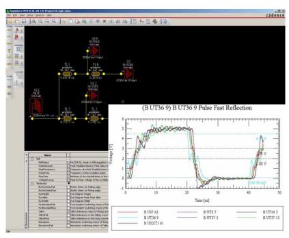
Figure 1: OrCAD Signal Explorer analyzes and validates topologies and interconnect to help minimize potential SI-related issues for fewer re-spins and shorter lab debug time
