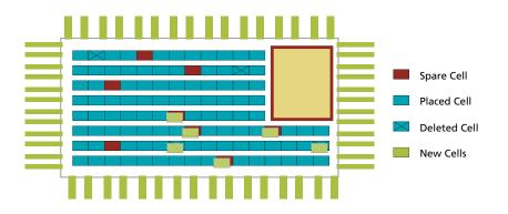
Figure 9: Design with ECO physically remapped
