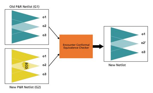
Figure 3: Conformal ECO Designer process diagram
