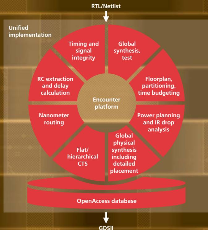
The Encounter platform is a full-chip, single-architecture RTL-to-GDSII system
