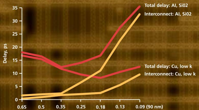
Wire delay exceeds gate delay at 0.18 micron and below in aluminum processes, and at 0.13 micron and below in copper
