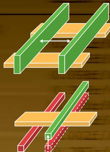
Timing and crosstalk are automatically calculated during routing and used to make on-the-fly decisions such as layer assignment and wire spacing
