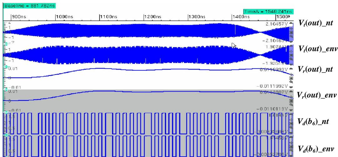
Figure 15. Partial waveforms obtained by normal transient simulation ( $V_t(out)_{nt}$ ,  $V_r(out)_{nt}$ , and  $V_d(b_6)_{nt}$ ) and local envelope simulation ( $V_t(out)_{env}$ ,  $V_r(out)_{env}$ , and  $V_d(b_6)_{env}$ ).
