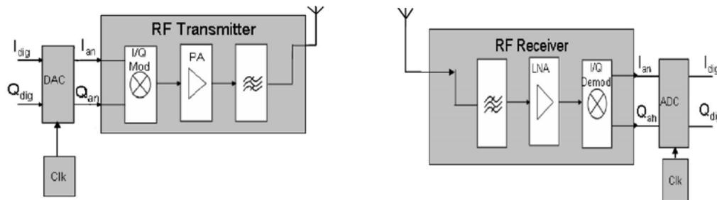
Figure 1. A typical RF transmitter and receiver for digital communication.
