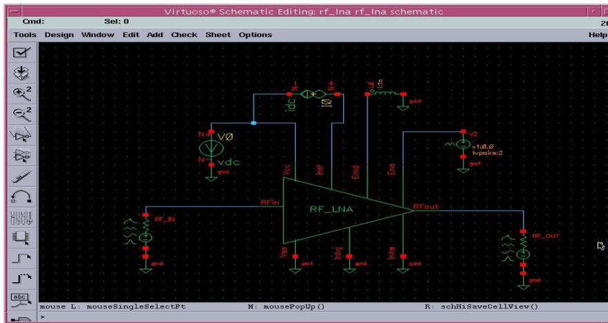
Figure 7. Schematic of the low-noise amplifier.
