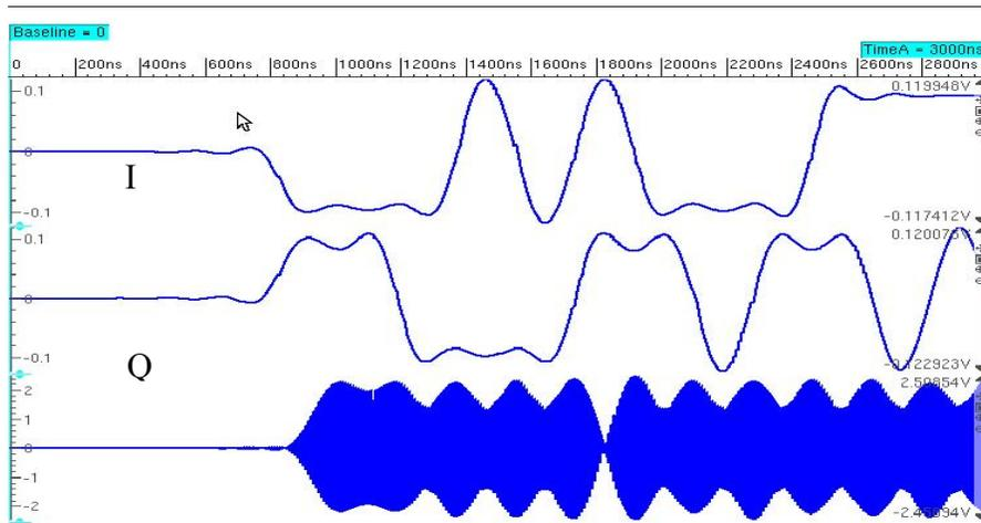
Figure 5. Typical I/Q and the composite signals from an I/Q modulator.
