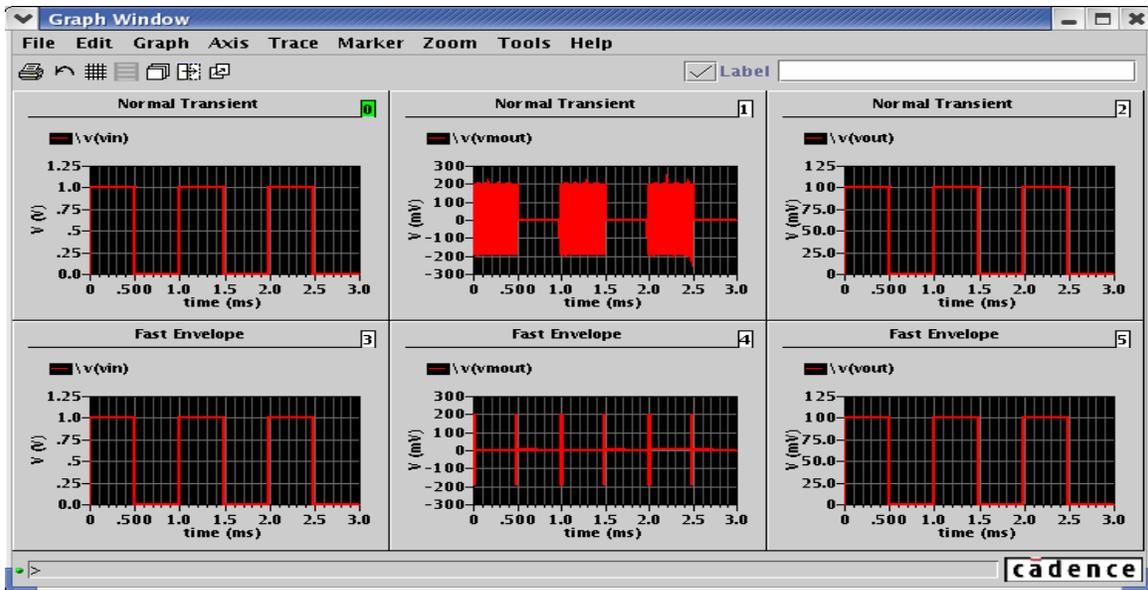
Figure 10. Input signal, modulated signal and output signal obtained by normal transient simulation (top ones) and fast envelope simulation (bottom ones).
