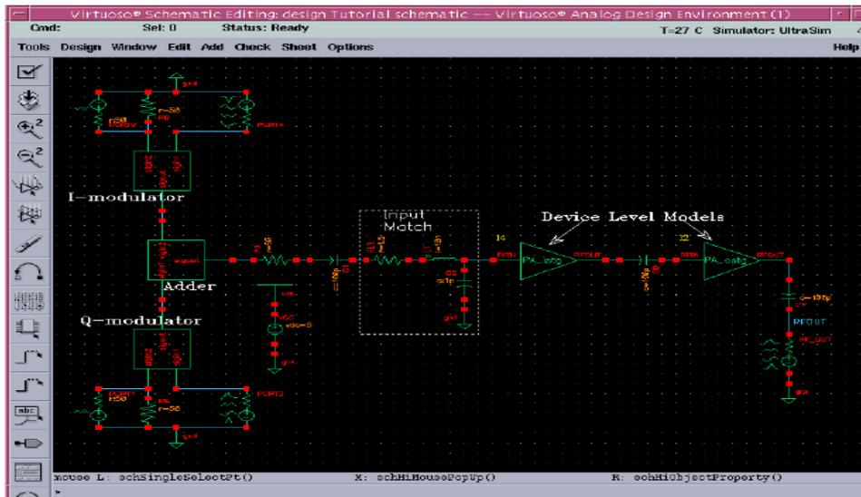
Figure 11. The schematic of a direct-conversion transmitter.
