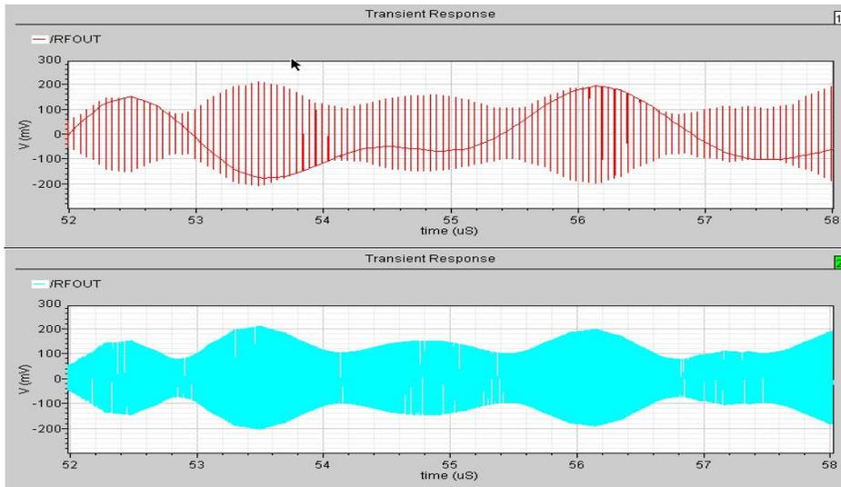
**Figure 12. The RF modulated signals obtained by fast envelope simulation (top part) and normal transient simulation (bottom part).**
