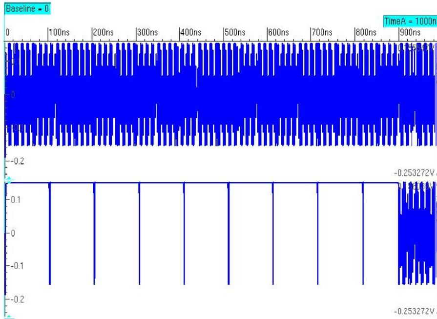
Figure 6. Waveforms obtained by normal transient simulation (the top waveform) and by fast envelope simulation for speed up (the bottom waveform).
