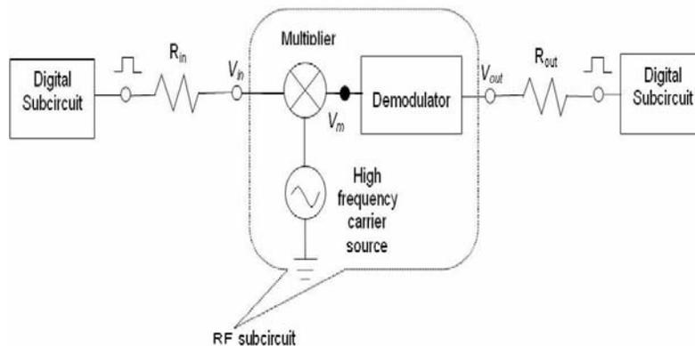
**Figure 4. A simple digital modulation circuit.**
