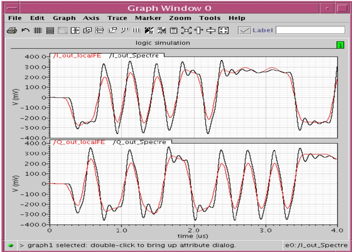
**Figure 17. The I/Q waveforms from Spectre transient simulation (in black) and UltraSim local fast envelope simulation (in red).**
