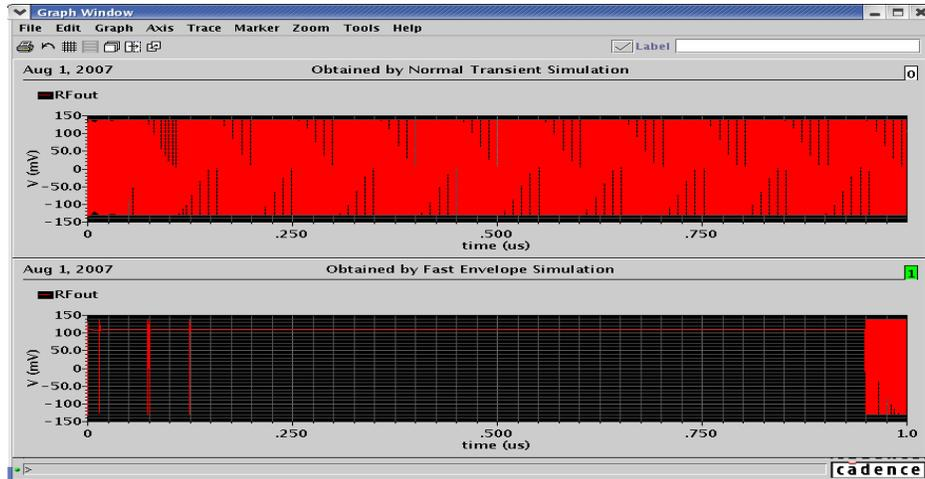
**Figure 8. RF output waveforms obtained by normal transient simulation (top part) and by fast envelope simulation (bottom part) of the low-noise amplifier.**
