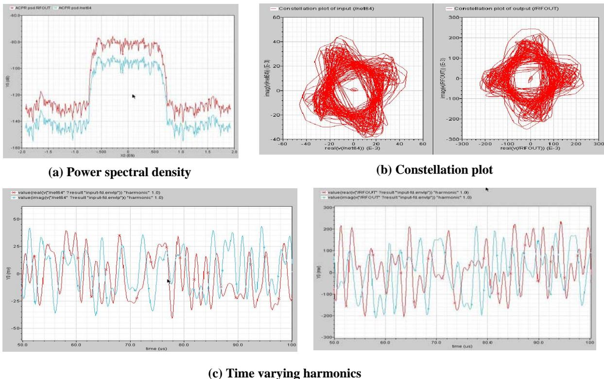
**Figure 13. Various plots of time varying RF characteristics.**
