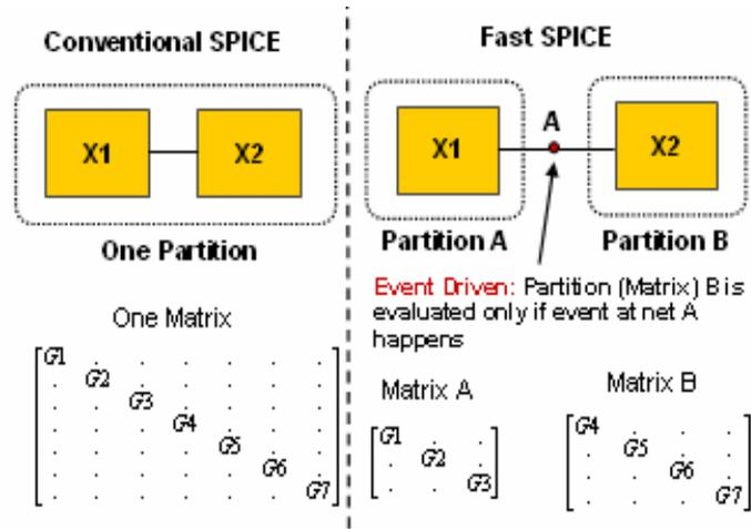
**Figure 3. A simple partition for FastSPICE simulation.**
