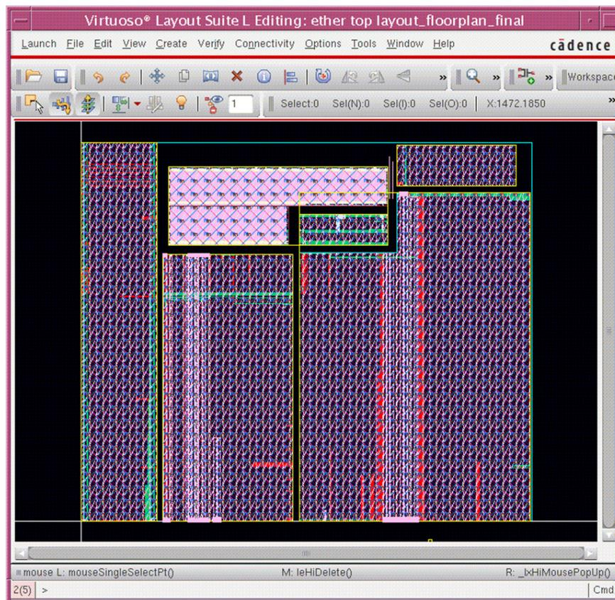
Figure 4. Floorplanning Block Placer
