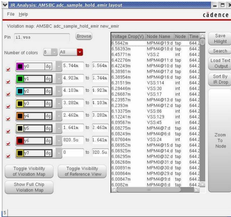
Figure 1.b) the user interface of IR analysis
