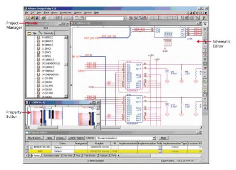
Figure 1: The multi-window interface of Cadence schematic capture technology simplifies navigation and searches across the hierarchy
