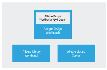
Figure 1: One Allegro Library Server is required per "site" or LAN; the PDM option connects to Allegro Design Workbench and enables work-in-process design data management and enhanced collaboration through Microsoft SharePoint 2010; the PDM option also provides integration with broadline third-party PLM solutions
