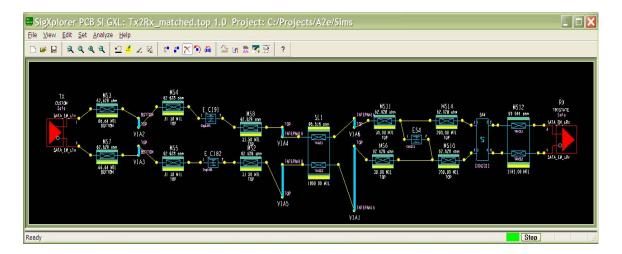
Simulating the SLOW corner shows a 7% improvement in the eye height margin, likely due to the loss improvement in the upper harmonics (as described earlier in the Route Analysis section), with the 250UI simulation now showing 337 mV.
