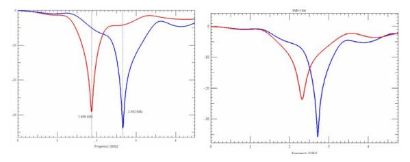
Routing the net with the ESD device in the series path (IC->ESD->Conn) we can remove the effect of the dangling stub. Now the insertion loss only reflects the LC of the ESD package/device. This is plotted next, along with the well-behaved loss we would see with the ESD device removed and the lengths matched (in green).
