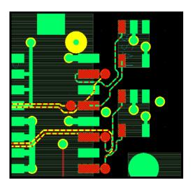
The energy in signals traveling through the nets will be divided between the connector path and the stub, causing a canceling of the signal when the stub is equal to a ¼ wavelength of the frequency. The length of stubs that will cause this problem are:
