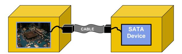
Since it is necessary to connect each board to the bulkhead connectors, additional cables and connectors are needed, as shown in the following diagram.
