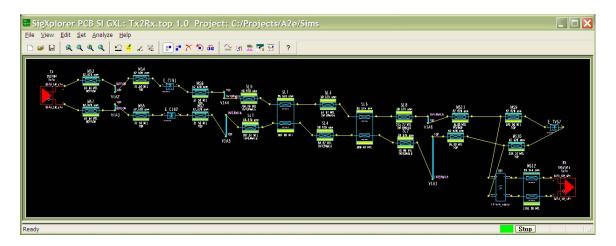
Note the behavioral "spec" MacroModels in red on the ends of the net, the PCB route extracted from the Controller board, the S-Parameter black box model of the cable/connector assembly, and the simple 3 cm trace to the Rx at the far end in the external drive.
