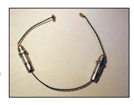
shows its loss is only about 1 dB down at 750 MHz, so we expect to see about 10% signal loss through the cable. At the higher frequencies observe how the assembly's reflected return loss dominates its transmission ability even as early as 2 GHz, so it would likely function poorly at higher rates. However, the transmission loss characteristic (S21) is basically linear up to around 1.8 GHz, so we have reason to be hopeful about the SATA signal behavior at 750 MHz.
