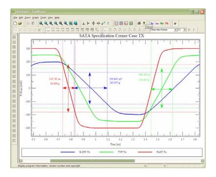
Transmit models with and without pre-emphasis were built to analyze performance against the various types of transmitters anticipated. The Tx models with ~10% pre-emphasis are shown at left. Note that pre-emphasis can only be seen when driving double-bits; the models will perform the same at the full data rate. The Tx models without pre-emphasis hold the specified levels constant (at right). Note that the slow corner is the same in both model sets in order to assess the worst case eye height.
