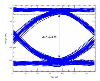
**Cable 1 Conclusions.** At 1.5 Gbps (750 MHz signal) this cable assembly shows acceptable loss. The interface functions decently as routed with the proposed cable, however the eye height is marginal. For better margin – and more importantly more predictable/reliable operation – use only Gen1m components and make the routing changes suggested in the Routing Analysis section.
