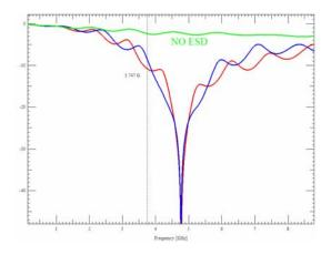
This frequency domain analysis suggests that the ESD devices should be routed in the series path to the connector rather than on a stub.
