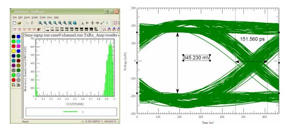
Checking the eye height at the slow corner follows the trend showing less margin due to the additional loss, with the slow corner (blue, at left) at 305 mV. As with Cable 1, Channel Analysis shows that this value holds across both 10k and 1 million bits (at right) at the SLOW corner since edges are slow and ringing is minimal.
