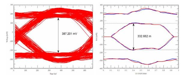
To further understand the signal behavior, remember that we're running "spec" corner models representing the edges of what might be seen using SATA compliant silicon devices. Looking at the corners we can see that the wider swings do press the limits of the 600 mV outer limit (see red waveform at left, FAST corner), yet the additional ringing induced by the fast edges causes the resulting eyes (at right) not to show as much
