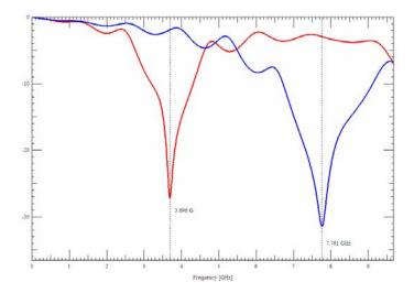
Doing the math we can derive the lengths of the stubs to be 400 mils and 190 mils, which is exactly the physical lengths of the two mismatched dangling stubs to the ESD devices.
