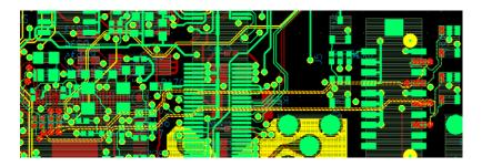
The SATA signals are shown highlighted in red. From the layout, note that the signals come off the IC pins (at left) through the AC capacitors and then route about 2 inches to the off-board PCB Connector connectors. ESD blocking components are farthest to the right and represent an additional load on the nets. The upper pair is the Tx signals, the lower diff-pair the Rx.
