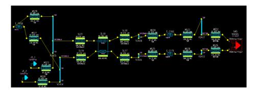
It was noted that the SATA diff-pairs on the Controller board could be routed with more precision (less skew), as can be seen in the various mis-matched lengths in the Tx and Rx paths. Using SigXp, it will be easy to quantify the improvement in signal quality if more careful routing is used.
