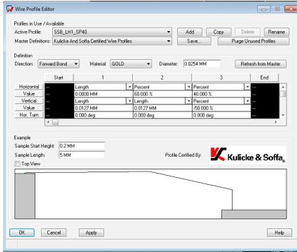
Figure 4: Includes a library of K&S-certified wire profiles optimized for their wirebonders.
