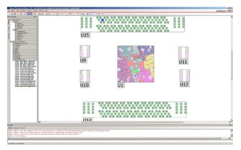
Figure 2: Placement/Floorplan view of the OrCAD FPGA System Planner provides users relative placement of critical components for optimum pin assignment synthesis
