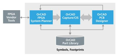
Figure 3: The OrCAD FPGA System Planner uses symbols and footprints from existing libraries
