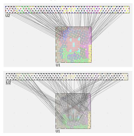
Figure 4: OrCAD FPGA System Planner optimization
